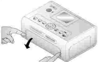
8. With the top paper tray cover open, insert the paper tray into the printer.
